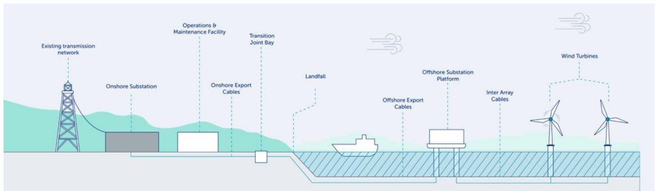
Figure 4.2: Main components of an offshore windfarm (OWF)
